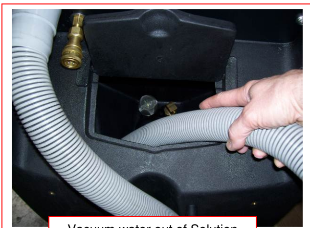
Vacuum water out of Solution Tank
